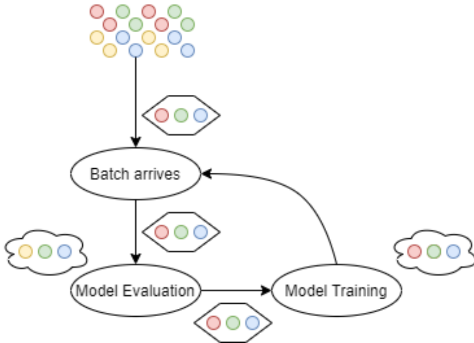
Figure 2.6: This figure demonstrates how interleaved chunks work, as it is almost like prequential, except it works in batches, depicted by the hexagons.
