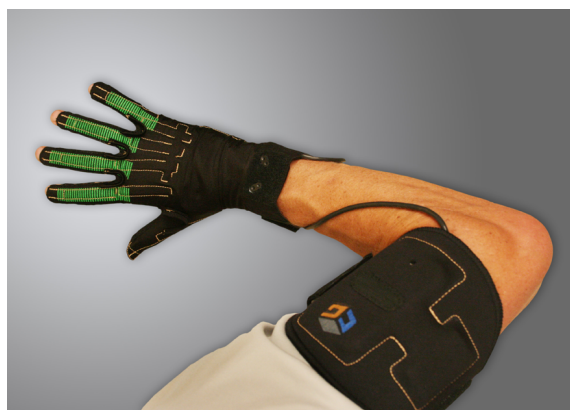
(a) CyberGlove Systems CyberGlove III
