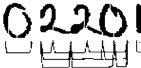
Figure 2-6 Example of a lattice and its possible segmentation paths (adapted from [NISHIWAKI & YAMADA, 1998])
