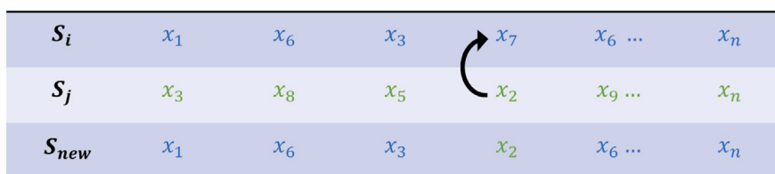
Fig. 3. Mutation process starts with two bags ( S_i and S_j ) drawn from the population. S_i has instance x_7 replaced by x_2 from S_j .
